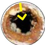
These pipes can cause discolored water, pressure issues and can corrode at the joints, which can lead to leaks. Galvanized pipes installed on water lines between 1880 and 1980 were dipped in molten, naturally occurring zinc. Naturally occurring zinc is impure, so these pipes were bathed in zinc that also contained lead and other impurities.
