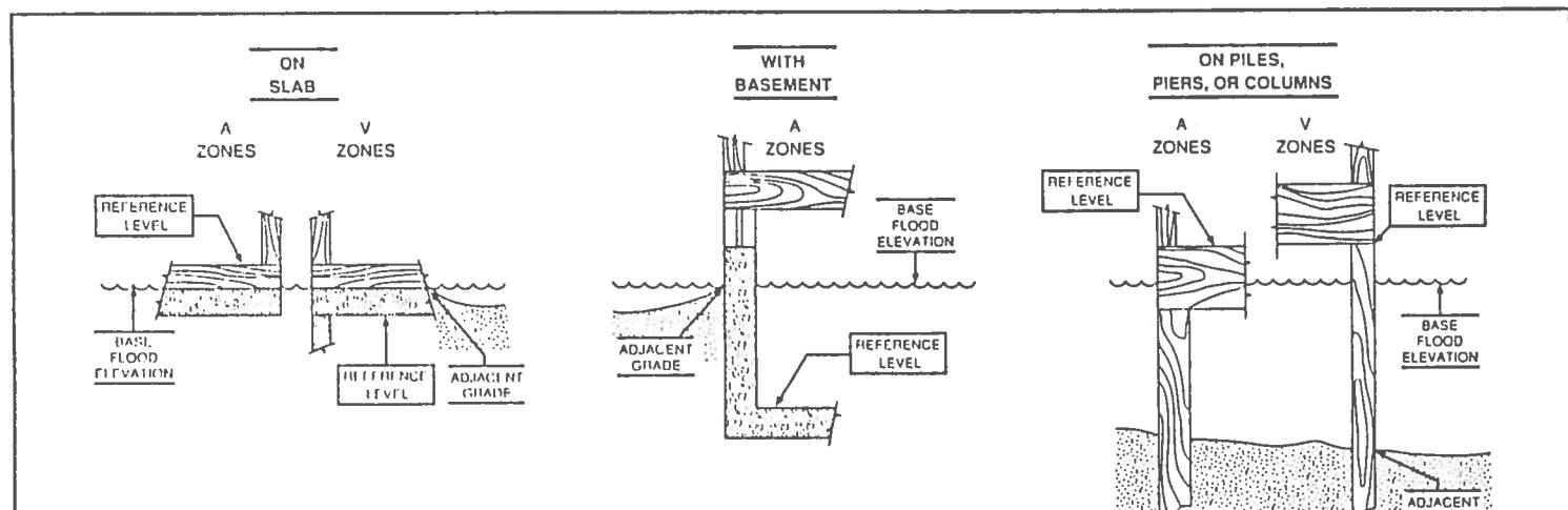
The diagrams above illustrate the points at which the elevations should be measured in A Zones and V Zones. Elevations for all A Zones should be measured at the top of the reference level floor. Elevations for all V Zones should be measured at the bottom of the lowest horizontal structural member.
