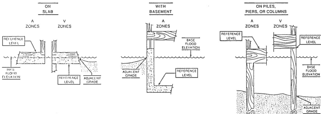
The diagrams above illustrate the points at which the elevations should be measured in A Zones and V Zones.
