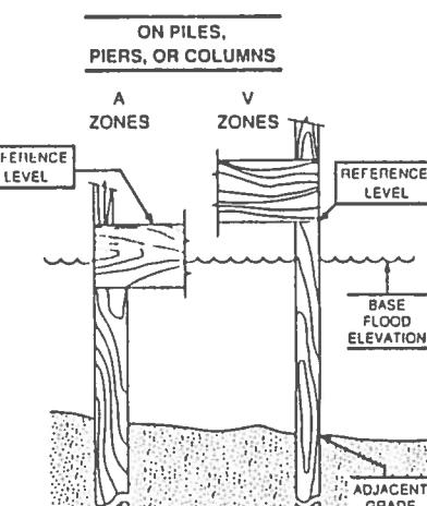
The diagrams above illustrate the points at which the elevations should be measured in A Zones and V Zones.
