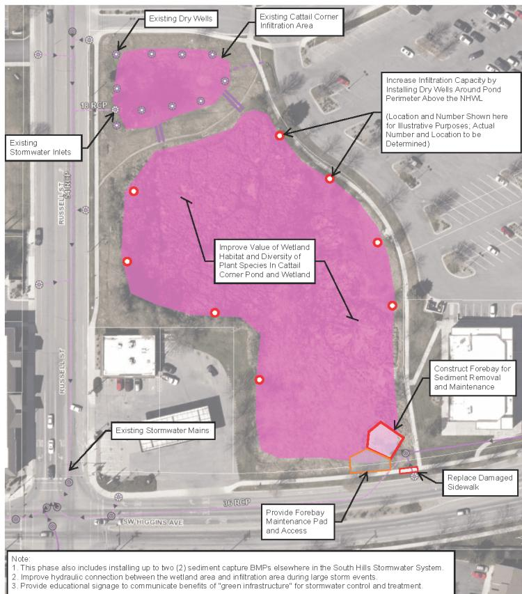
**Description:** This phase of the South Hills Stormwater Project will improve how Cattail Corner functions as a stormwater treatment wetland. Additional work will be done to offset increased flows to the storm drain system due to the Gharrett Street Project.
